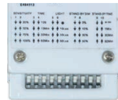
Sensor Dip Switch Settings (Dip Switches on Sensor)
